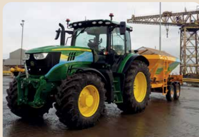
JOHN DEERE 6155R TRACTOR WITH TOWABLE GRITTER
